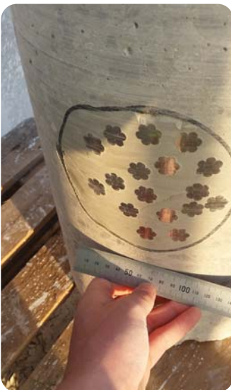
Core sample of void-free section showing cable tendons surrounded by Cable Grout
